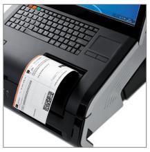
AUTOMATIC SCANNER ACTIVATION when a document is inserted
